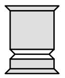
Starting with the wooden spool, you'll need to create a groove around the base. A V-shaped tool on the lathe works well for this operation. You'll also need to drill a 3/8 inch (9 mm) hole 2 inches (51 mm) deep into the top end of the spool for the feathers.
